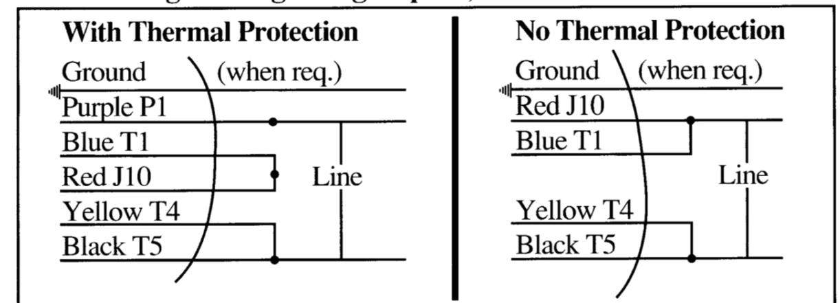
Connections shown are for CCW rotation viewing lead end of motor.
